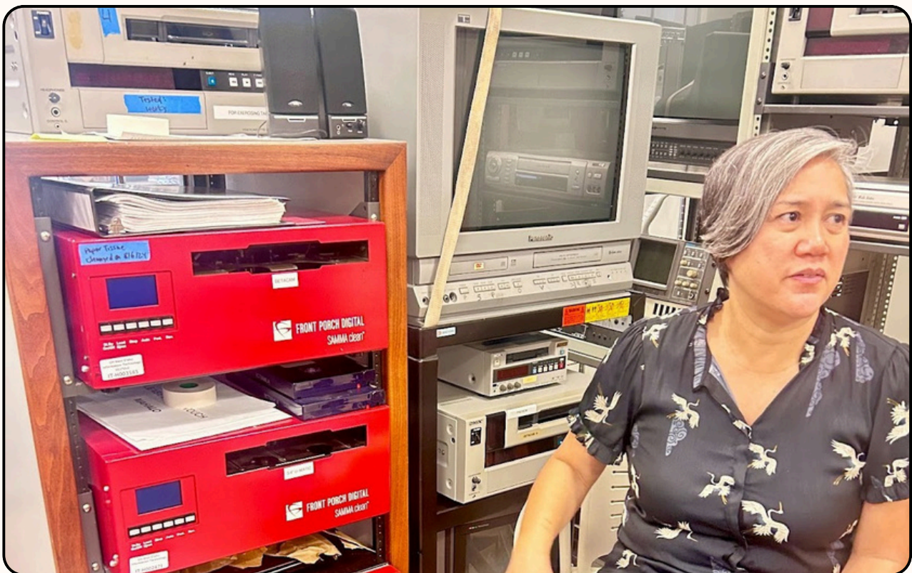
Above: Janel with the U-matic tape cleaning machine and a Beta tape cleaning machine. These were part of the organization's SAMMA system, and are the only part of the system still in use.
