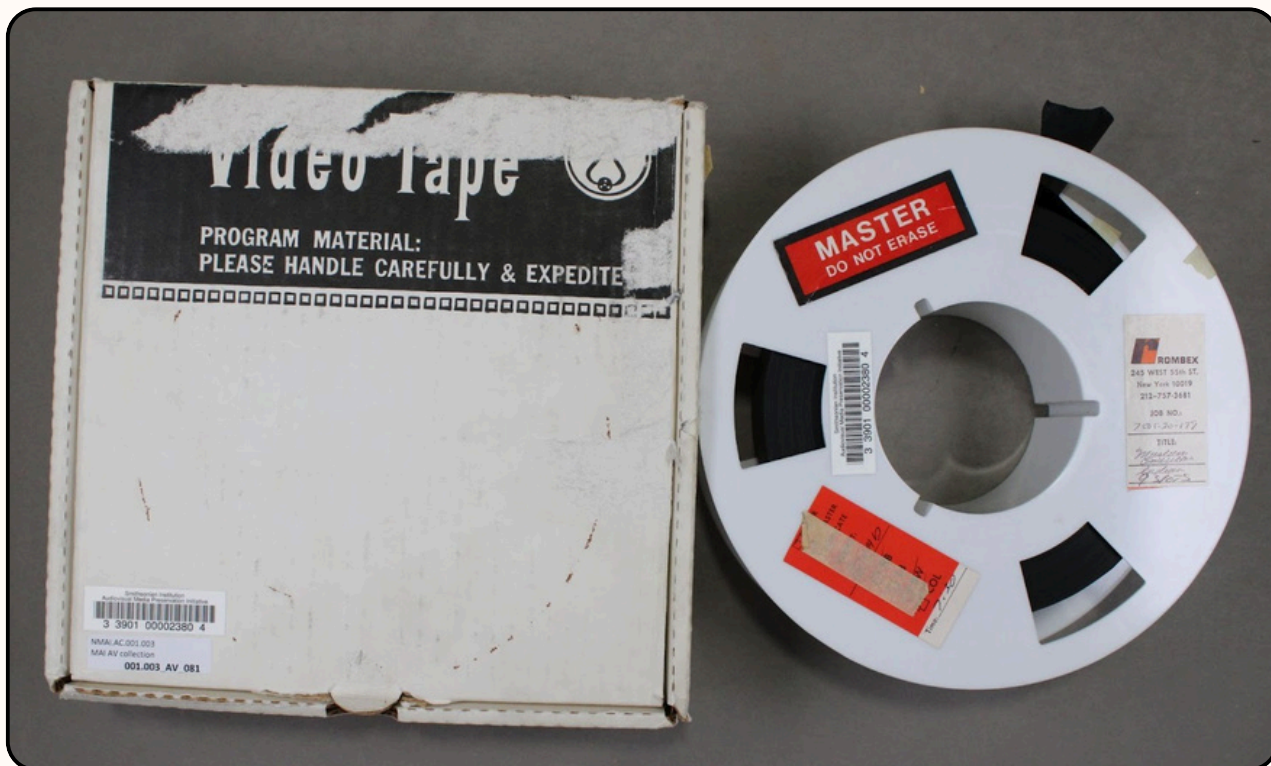
Above: A 2" quadruplex videotape television commercial from the National Museum of the American Indian (NMAI). Object # NMAI_001.003_33901000023804_p. Digitizing 'degrading' magnetic media formats are a preservation priority for AVMP, and the initiative has eliminated 2" quadruplex analog videotape and D-2 digital videotape formats from its list of un-digitized 'at-risk' formats across all SI collections.
